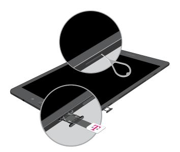
**Caution**: Exercise care when using the metallic removal tool to eject the internal SIM card slot.
