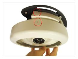
**NOTE:** The cables must be slightly bent underneath the cover ring.
