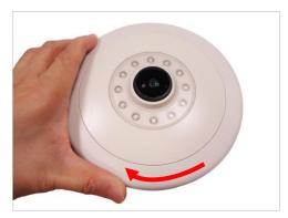
4. Remove the thin film protecting the lens.
