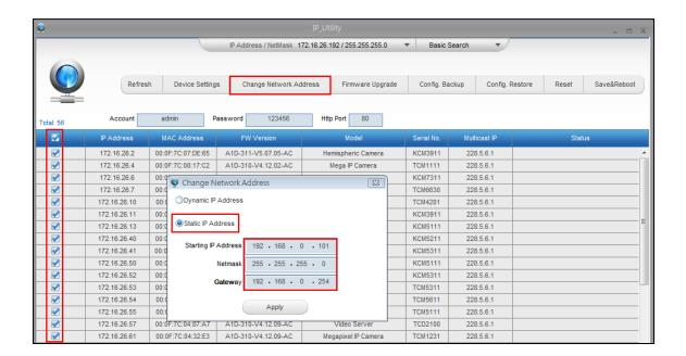
With the procedure shown above, all the cameras will have unique IP addresses, starting from 192.168.0.101. In case there are 20 cameras selected, the last one of the cameras would have the IP 192.168.0.120.
