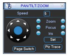
On both control panels there are controls for zoom, focus and iris (light level). The QD6531Z has a 3x optical zoom lens which will adjust between 5 and 15mm. The camera has an autofocus feature and is not user adjustable. Objects closer than 20" (50cm) will be blurry due to the limits of the automatic focus. Likewise, the camera automatically adjusts the iris internally and that setting is not manually changeable by the user.
