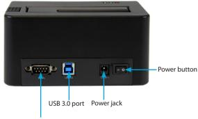
RS232 serial-based printer port
