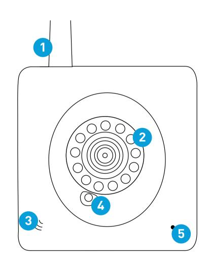
1) Audio Out: To use the intercom function, connect speakers to the audio output. Using the mobile app, you can talk to your mobile device and your voice will be heard on the speakers connected to the camera.
