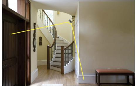
Have a look at the image(s) on the DVR/NVR first before installing the cameras permanently.
