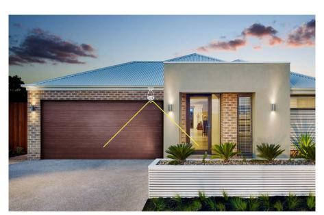
Install the camera where the roof meets the walls — of the house.
