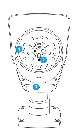
1) Wi-Fi Antenna: The included Wi-Fi antenna connects to the camera here.
