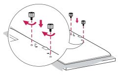
3 Use the screws to secure the stand to the back of the product as shown below.
