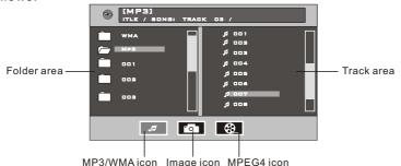
During MP3/WMA playback, the root menu above displays all the time.
