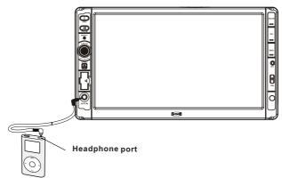
2. Play the external iPod, then use SRC button to enter AUX IN mode for the car AV system. By now, the program played by the external iPod can be output through the monitor of the car AV system and the speakers connected to the car AV system.
