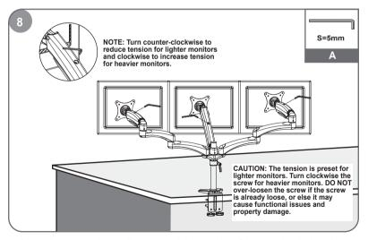
Use a hex wrench to adjust the height tension of the mechanical spring arm, to keep different weight of monitors still at any position.
