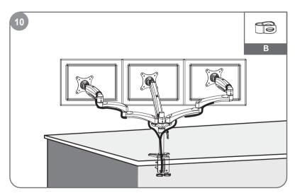
Insert cables into cable covers. Leave enough slack of cables at arm joints for full adjustment.
