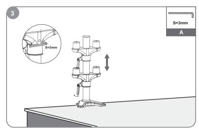
Adjust locating ring at proper height and screw up tight to hold the mount. Adjust aluminum support part above the locating ring and use a hex key to fix it.
