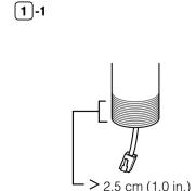
Pass necessary cables for connecting the camera through the pipe.
