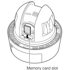
Remove the dome case and place the memory card in the memory card slot.
