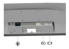
3. Connect one end of the analog signal cable to the monitor D-SUB connector and the other end to the computer.
