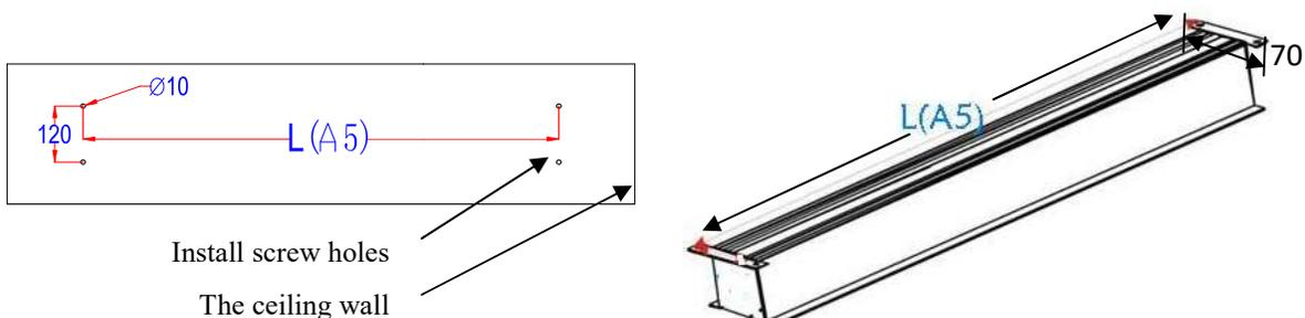
3. The **M8expanding bolts (G)** mount into thick wood beams, stone or concrete and will support the screen. Use the **Socket wrench (D)** to attach the **M8x40mm hexagonal screws (H)**. The expanding bolts should be firmly tightened and tested to make sure that they will hold the weight of the screen.
