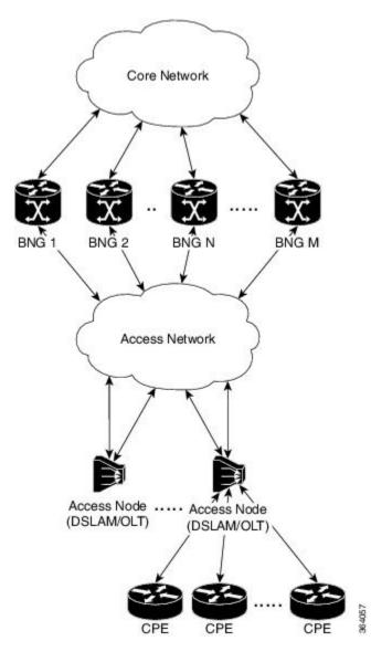
The redundancy pairing between BNG routers work by synchronizing the state from the master (active) to the slave (backup).
