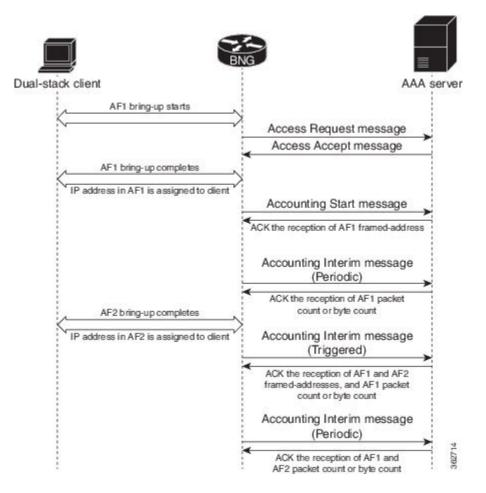
The details of the call flow between the BNG router and the AAA server are listed here:
