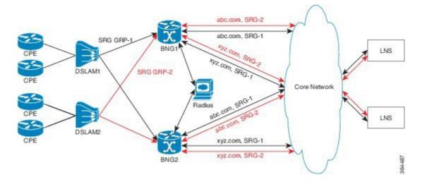
For a PPPoE-LAC geo redundancy setup, the SRG is formed by grouping together the access-links on which LAC sessions are to arrive (co-exists with PTA). To enable SRG level redundancy switchover, tunnels for
