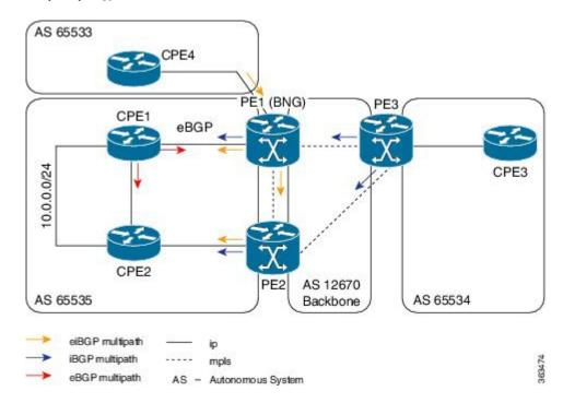
All Provide Edge (PE) routers shown in the figure, are in the service provider Autonomous System (AS), representing the core of the network. The CPE1 and CPE2 are in customer AS, peering with the PEs (PE1 and PE2 respectively) as eBGP neighbors. A statically-configured loopback address on CPE and PE, is used for BGP peering. There are networks behind the CPE, and the CPE advertises respective prefixes to the PE routers through eBGP.
