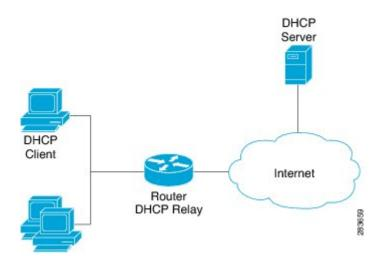
The DHCP server allocates IP addresses for only a configurable period of time known as the lease period. If a client device needs to retain the IP address for a period longer than the lease period, then the client must renew the lease before it expires. To renew the lease, the client sends a unicast request to the DHCP server. On receiving the request message, the server responds with an acknowledgment, and the client's lease is extended by the lease time specified in the acknowledgment message.
