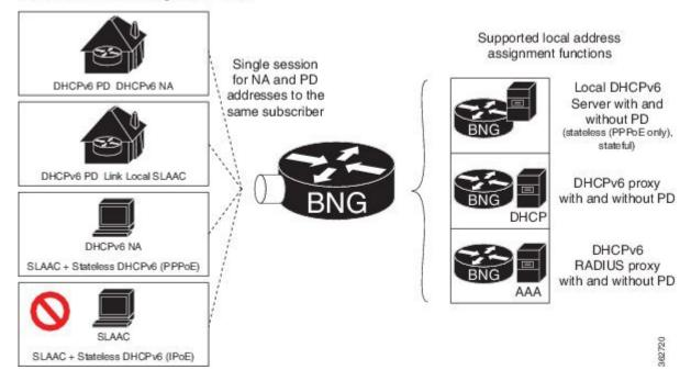
Cisco ASR 9000 Series Aggregation Services Router Broadband Network Gateway Configuration Guide, Release 6.0.x The **framed-ipv6-address** RADIUS attribute can also be used to provide an IP address from the RADIUS server to the subscriber. This address is then advertised through a Stateless Address Auto Configuration - Neighbor Advertisement or Neighbor Discovery (SLAAC - NA or ND) message for both PPPoE and IPoE sessions.
