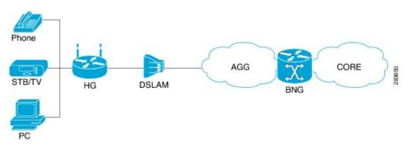
In the Network Service Provider model, the ISP (also called the retailer) directly provides the broadband connection to the subscriber. As shown in the above figure, BNG is at the edge router, and its role is to connect to the core network through uplinks.
