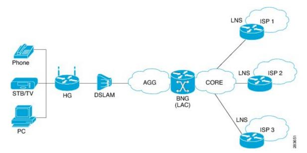
In the Access Network Provider model, a network carrier (also called the wholesaler) owns the edge network infrastructure, and provides the broadband connection to the subscriber. However, the network carrier does not own the broadband network. Instead, the network carrier connects to one of the ISPs that manage the broadband network.
