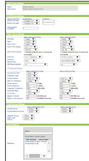
In addition to this topology, each Access Point Group can override settings from the Default System Group and each Access Point can override settings from the Access Point Group that it belongs to.
