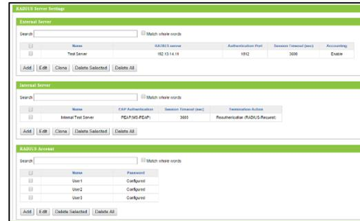
A RADIUS Group can have a 2.4GHz Primary and Secondary RADIUS Server. In addition 5GHz Primary and Secondary RADIUS Servers can also be assigned to the RADIUS Group. Members for the RADIUS Group can then be added as well.
