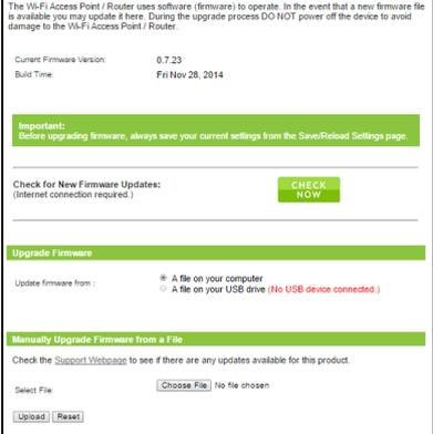
The Wi-Fi Access Point / Router uses software (firmware) to operate. In the event that a new firmware file is available you may update it here. During the upgrade process DO NOT power off the device to avoid damage to the Wi-Fi Access Point / Router.
