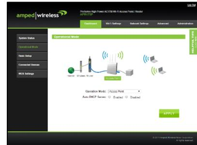
Basic setup will detect your network settings and automatically configure the Access Point to your network.
