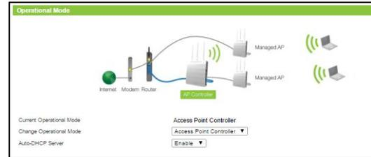
The Auto-DHCP Server feature automatically manages the IP addresses within your network. When connected to a network that has a DHCP server enabled, the Access Point/Router will automatically obtain an IP from the network's DHCP server and disable the DHCP server on the Access Point / Router to avoid any IP assignment conflicts. For users that are not familiar with how this works, it is recommended to leave Auto-DHCP server enabled on this page.
