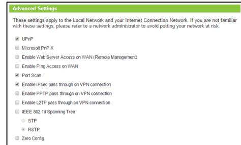
Enable IPsec pass through on VPN connection: Allows the IP security protocol suite to pass through on a VPN connection.
