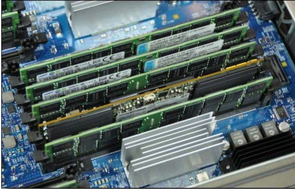
Figure 5. eXFlash DIMM installed in the Compute Book
