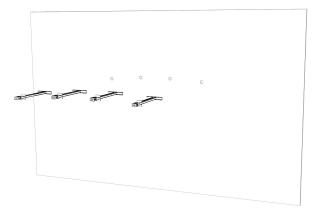
4. Place wall mounting bracket over flanges and install 1/4"-20 bolts to affix bracket to the wall.
