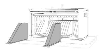
8. Install two screws (included) to secure the unit to the surface mounting bracket.
