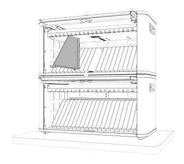
13. Install two screws (included) to secure the upper unit to the stacking bracket.
