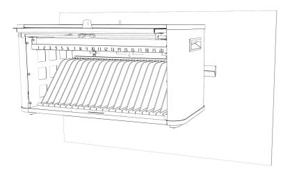
Install two additional bolts via the front of the PureCharge Station™ to secure the unit to the wall mounting bracket.
