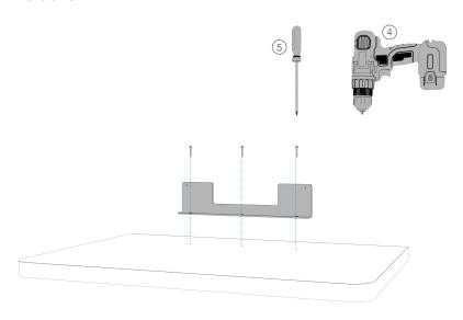
5. Secure the bracket to surface with appropriate fasteners (not included).
