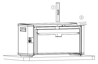
3. From the front, install the remaining two self-tapping screws to secure the stacking bracket from the inside of the station.
