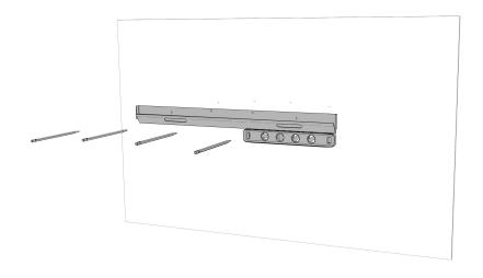
2. Drill ½" diameter holes. If using the included hollow wall fasteners, locate holes in clear space between studs.
