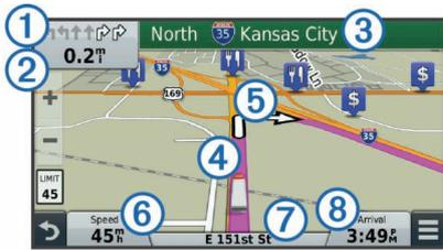
Instructions for your next turn or exit, or other action appear across the top of the map. The symbol ① indicates the type of action and the lane or lanes in which you should be traveling, if available. The device also displays the distance to the next action ② and the name of the street or exit associated with that action ③.
