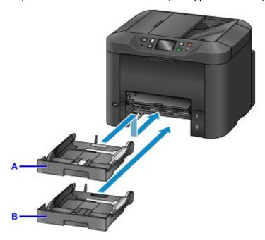
In the upper cassette 1 (A), all sizes of paper compatible with this machine (plain paper, photo paper, envelopes, etc.) can be loaded.
