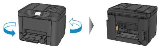
2. If the protective material for the rear cover remains attached, remove it.
