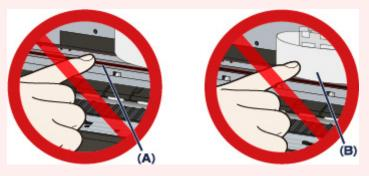
If the paper or your hands touch these parts and blot or scratch them, the machine can be damaged.
