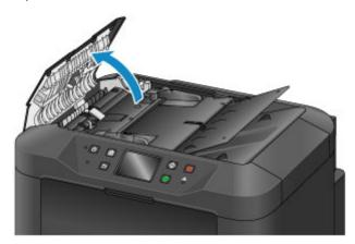
3. With the clean cloth, wipe off any paper dust from the inside of the document feeder cover (A).
