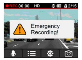
**G-Sensor event recording:** During video recording, if the DrivePro detects an impact, it will automatically activate emergency recording mode.
