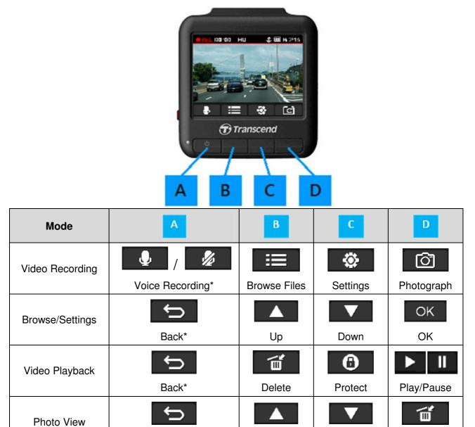
\*Press and hold for 3 seconds to turn on/off the DrivePro in any mode.
