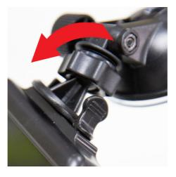
**5.** When the DrivePro is in the best position, turn the adjustment knob clockwise to make sure the DrivePro is securely locked in place.
