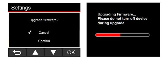
WARNING: NEVER remove the power cord or the microSD memory card while the firmware is being upgraded.
