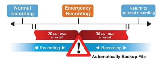
**Manual event recording:** During video recording, press the emergency button on the left-hand side of the DrivePro to manually activate emergency recording mode. The emergency icon will appear on the screen when activated.
