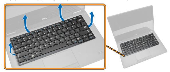
**4.** Lift up to remove the keyboard trim from the computer.
