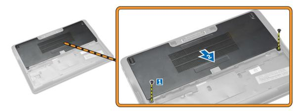
**4.** Lift the base cover to remove it from the computer.
