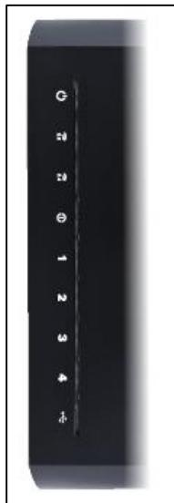
**Power:** Indicates when the Router is powered on. The LED will remain on.
