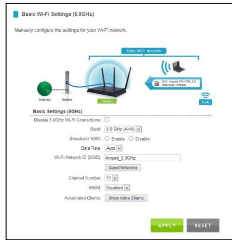
**Wireless Network ID (SSID):** The name of your 5GHz wireless network.
