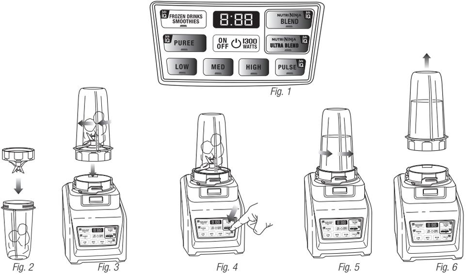
**NOTE:** Nutri Ninja® | Ninja® Blender Duo™ with Auto-iQ™ Technology can sense which jar is on the motor base. The available function lights will illuminate depending on which jar is placed on the motor base. (Fig. 1)
