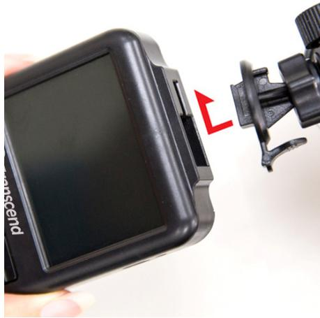
2. Thoroughly clean and dry the area of the windshield you wish to mount the DrivePro. If possible, mount the DrivePro in the middle of the windshield near the rear-view mirror for the best field of view.
