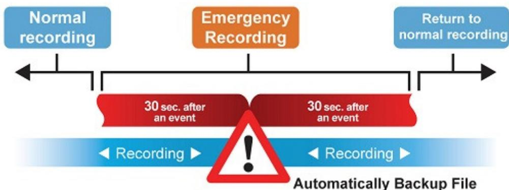
**Manual event recording:** During video recording, press the emergency button on the left-hand side of the DrivePro to manually activate emergency recording mode. The emergency icon will appear on the screen when activated.
