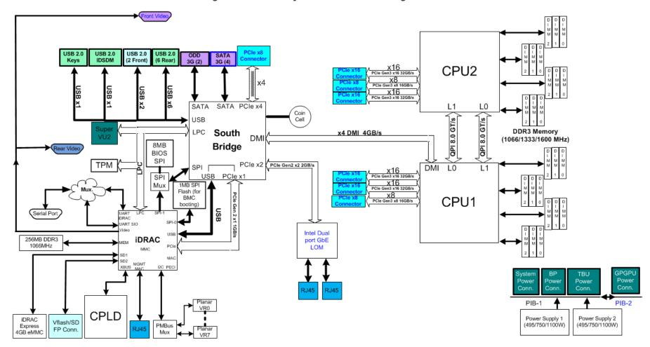
Figure 14. T620 system board block diagram
