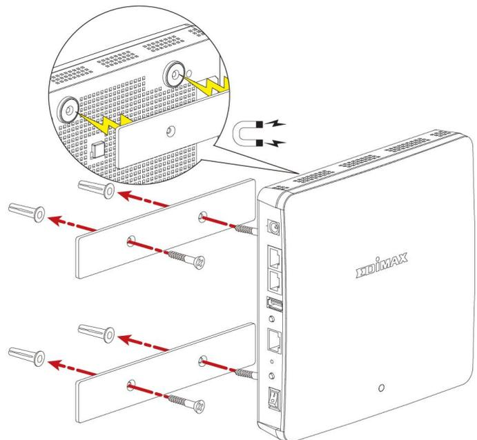
3. Press the back of your access point firmly against the two wall mounted magnetic strips, with the access point's Edimax logo in the correct, upright orientation as displayed above.
