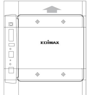
2. Attach the two magnetic wall mount strips to your wall using the included screws, as shown below.
