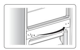
9. Place refrigerator flatwise, remove part③ and then loose screws④. Remove part ② and part①.
