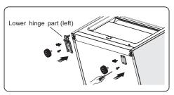
12. Move the lower door and adjust its position to align lower hole site and upper hinge axis. Turn the middle hinge by 180, change the washer on the axis to the upper side, adjust the middle hinge to the appropriate position and then install it.
