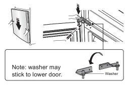
13. Screw out The upper hinge axis, turn the upper hinge over and fix axis on it. Then place it at side for use.
