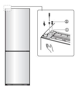
15. Install part the upper hinge cover (which is in the plastic bag).
