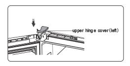
16.Reverse part① by 180° and install it onto the right corner of upper door, then mount part②. (both of which are taken down in step 2)
