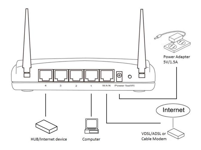
4. Check all LEDs on the front panel. The PWR LED should be steadily on; the WAN and LAN LEDs should be on if the computer / network device connected to the respective port of the router is powered on and correctly connected. If the PWR LED is not on, or if any LED you expect to be on is not, recheck the connections or refer to 4-2 Troubleshooting for possible reasons and solutions.
