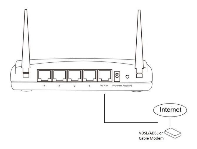
2. Connect all your computers, network devices (network-enabled consumer devices other than computers, like game consoles or switches) to the LAN port of the router.
