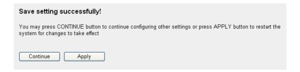
Click Continue to go back to the previous setup menu or to continue to other setup procedures; or click Apply to reboot the router so the settings will take effect (wait about 40 seconds while the router is rebooting).
