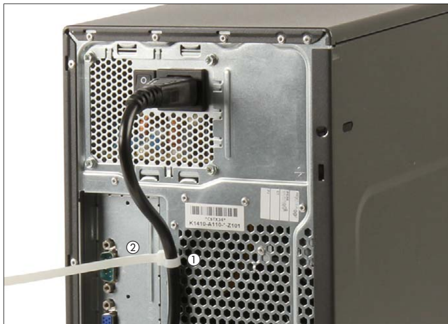
Figure 3: Securing power cord
