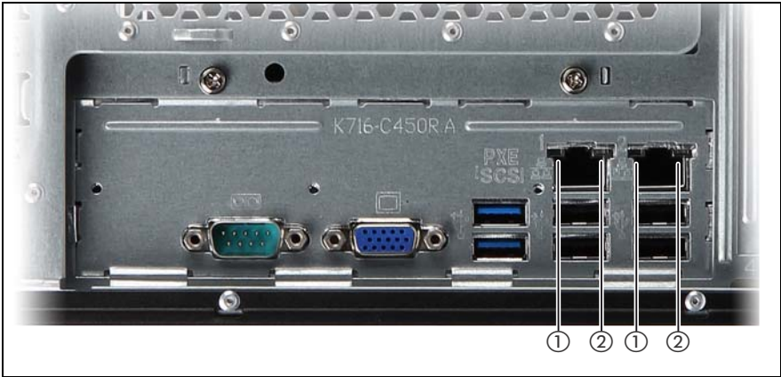
Figure 6: Indicators on the connector panel: LAN indicators
