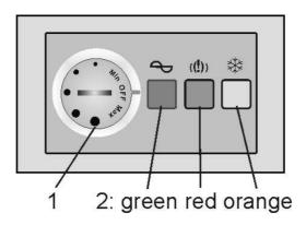
The indicator light set is placed on the front side of the freezer for easy visibility.
