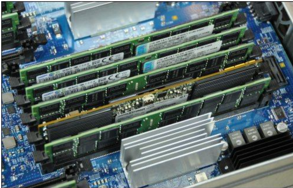
Figure 5. IBM eXFlash DIMM installed in the Compute Book
