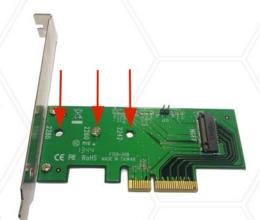
Step 2. Insert a PCI Express M.2 media card into the slot at an angle.
