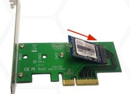
Step 3. Gently hold down the media card while securing it with the screw.
