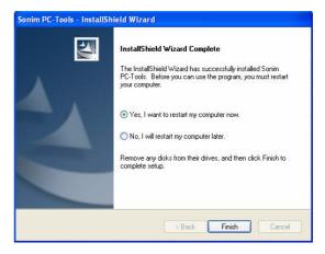
Select the suitable restart option and click Finish to complete the installation process.
