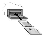
There are pay TV services available; these are accessible with the use of a Conditional Access Module (CAM) and a subscription card. A Common Interface (CI) is the slot into which you can insert a CAM. The front of the digital receiver has two common interface slots. To watch a pay service, you should take the following steps:
