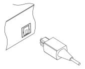
To enjoy Dolby Digital audio, your television or audio-video receiver must be able to decode Dolby Digital audio, and you need to obtain an S/PDIF cable. Plug one end of the cable into the S/PDIF socket on the digital receiver, and plug the other end into the matching socket on your audio-video receiver.
