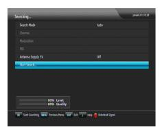
To perform service search, select the Installation > Searching menu. You should see a screen like the left figure. If you have an antenna booster, you should set the Antenna Supply 5V option to On to supply power to it.
