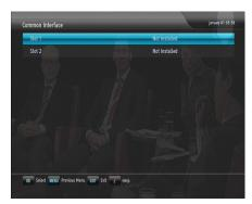
To view the information about the module and subscription card which is inserted into the digital receiver, select the Common Interface menu.
