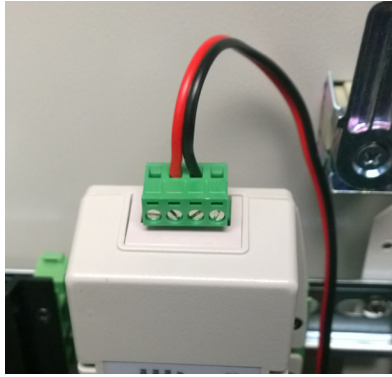
Green Terminal Connector attached to Power Injector
