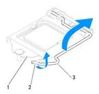
1 processor cover 2 tab 3 release lever
