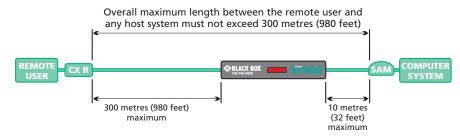
In situations where any computer system will be placed a significant distance from the ServSwitch CX Uno unit, ensure that the distance to any remote user is similarly less than 300 metres (980 feet).
