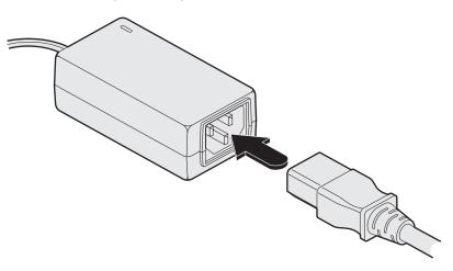
3 Connect the power lead to a nearby main supply socket.
