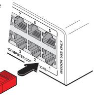
3 Connect the other end of the cascade link cable to the remote user RJ45 socket on the front panel of the lower unit.
