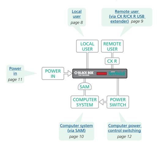
Connections do not need to be carried out in the order given within this guide, however, where possible connect the *power in* as a final step.
