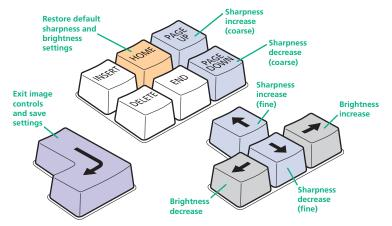
3 When no shadows are visible and the displayed images have crisp edges, press [1] to exit configuration mode and permanently save all settings. The new compensation settings will be stored, even when power is removed or if a complete reset is initiated. These settings should not require further changes unless the cabling arrangements are altered.
