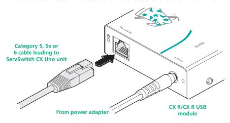
5 At the other end of the cable run, attach the cable connector to the socket on the front panel of the ServSwitch CX Uno unit.
