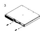
1. Remove two screws and right side front panel.
