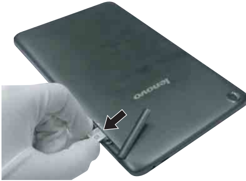
Figure 2. Removal steps of Micro SD card and Micro SIM card (continued) Pull out the SD card or SIM card from its slot.
