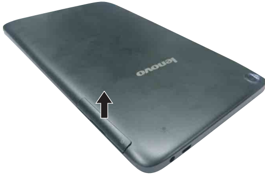
Figure 2. Removal steps of Micro SD card and Micro SIM card Insert a finger to open the side door as shown in the picture.
