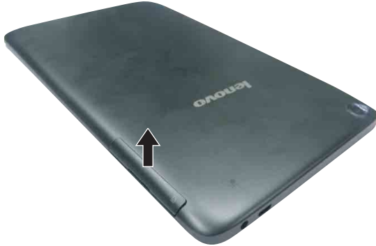
Figure 3. Removal steps of back cover
