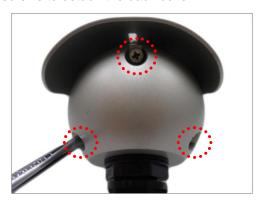
**NOTE:** A cable is connected inside the camera; do not abruptly pull the back cover.
