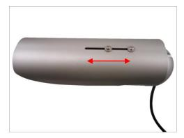
3. Tighten the screws to fix the position of the sunshield.
