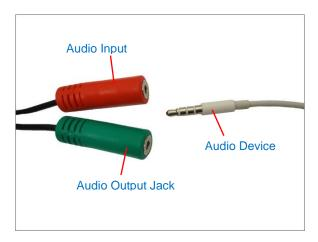
**Note:** Make sure that the connected audio input device has a built-in amplifier. Connecting an ordinary microphone will dwarf sounds and will result in inaudible recording.
