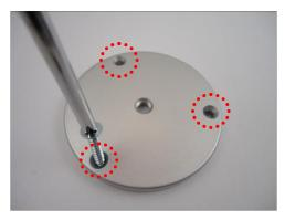
3. Attach the bracket to the plate.
