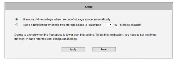
Please note that under this mode, there is a risk that important evidence may be deleted automatically over a period of time. Therefore, as long as "recycling" mode is used, the user should download the critical evidence files from the camera before they are erased by the camera.
