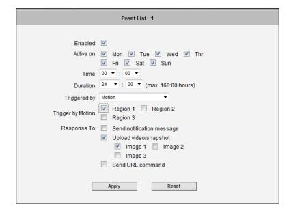
By the example above, the camera will be 24/7 on guard to watch for motion events. When motion detection region 1 detects intrusion, it will trigger the response of uploading "image 1" according to the parameters defined under "Event Configuration" earlier. In other words, whenever motion occurs, the camera will record 3 seconds of video before the moment of motion detection, and 57 seconds after that. The video file can then be found under "Local Storage" -> "File Management".
