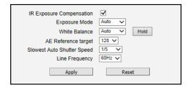
**IR Exposure Compensation** is available on all cameras with IR ILEDs. This feature automatically balances the IR exposure to eliminate over-exposed images cause by too much IR on the subject. When enabled, the AE reference target is automatically adjusted to control the sensor's shutter speed and gain to compensate IR effect.
