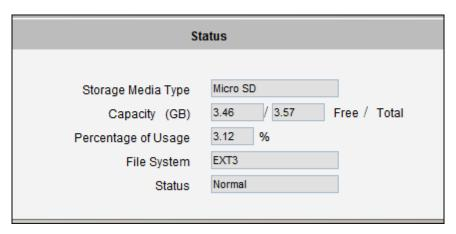
In case of IP cameras with installed memory cards, the Storage Media Type will show "Micro SD".
