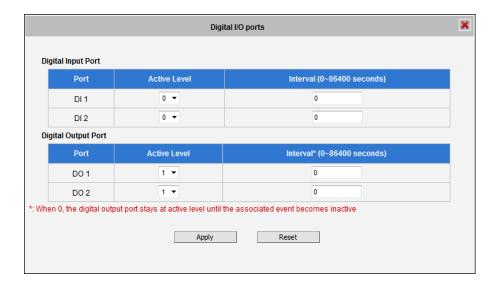
The Digital I/O Ports page displays the number of available DI and DO ports on the camera, which varies depending on camera model.
