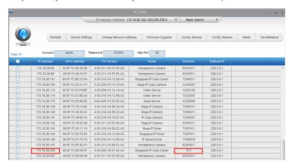
You can quickly notice the **D11** model in the list. Click on the IP address to automatically launch the default browser of the PC with the IP address of the target camera filled in the address bar of the browser already.
