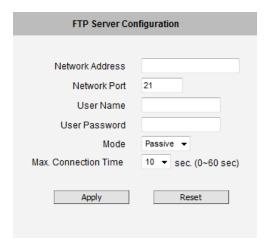
To setup FTP servers, make sure to enter the network address of FTP server, the Network (FTP) port, the User Name and Password of FTP account, Connection mode (Passive or Active) and Connection time before timeout.
