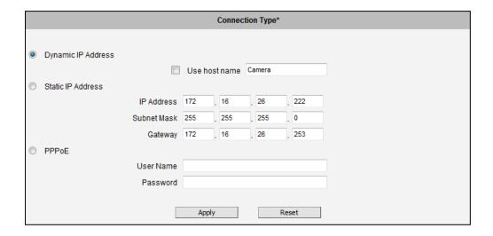
**Host Name** is used to identify the camera by a DHCP server. In some networks with very strict security policy, it is required that all the network devices should have their host name, and when the devices attempt to access the network by requesting an IP address from a DHCP server, the DHCP server would check if the host name is among the allowed devices. On this page, it is possible to edit the Host Name and enable or disable the use of host name.
