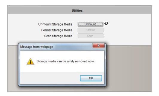
That Unmount function is used when the camera is to be shut down for maintenance or when the mass storage has to be physically removed for some reason. The purpose of unmounting is to protect the currently processed data on mass storage at the moment of removal of the storage. If
