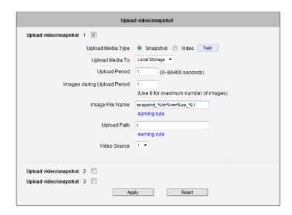
With the settings above, it would create 1 snapshot within 1 second from the moment of triggered event using following file name snapshot\_%YYYY-%MM-%DD-%hh-%mm-%ss.
