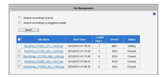
The largest possible recording file is approximately 30 minutes. You can see the length of each file in the file list. In case of snapshots, the length is 0.
