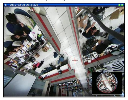
If Miniature Fisheye-view is enabled, the current direction and scope of view is shown on the Miniature Fisheye-view window with the red marking.
