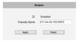
Similarly to UPnP, the human readable **Friendly Name** can be defined by the user. That name will be displayed when the camera is found in the network. By default, the Friendly Name is the serial number of the camera; however, the user can modify the name according to the project needs.
