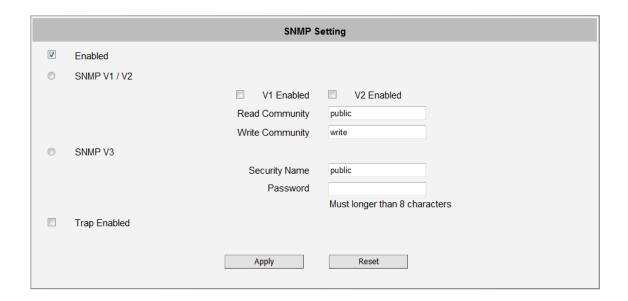
The SNMP agent supports versions V1, V2 and V3. SNMP V1 is the initial implementation of SNMP. SNMP V2 is proposed to enhance the performance of management, such as the communication of server and devices, the confirmation of information delivery and receipt. Primary additions in SNMP V3 concern security and remote configuration enhancements.
