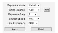
In manual exposure mode, the user can directly adjust the signal gain and shutter speed manually. The White Balance and Line Frequency controls have already been explained in the previous chapter.
