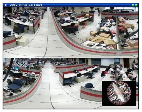
If Miniature Fisheye-view is enabled, the current scope of view is shown on the Miniature Fisheye-view window with the red marking.
