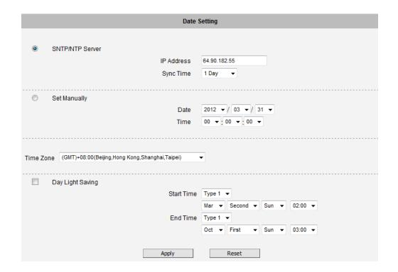
When choosing **SNTP/NTP Server** for automatic date and time updating, you can key in the IP address of the NTP server and the time interval for automatic time synchronization. If you want to key in the domain name of NTP server instead, please make sure the DNS server IP address has been set under IP Settings; otherwise the camera will not be able to resolve the domain name of the NTP server.
