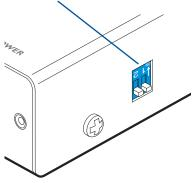
Figure 3-6. Power derivation switch
