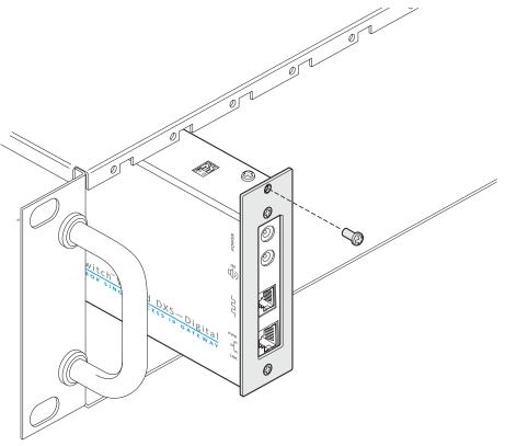
Figure 3-2. Fixing the module into the rack
