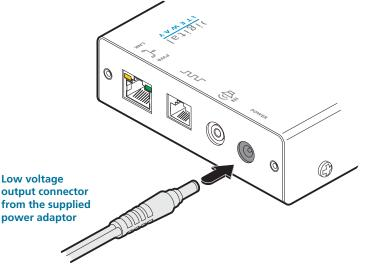
Figure 3-7. Connecting the power adaptor
