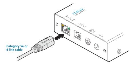
Figure 3-5. Connecting a network cable
