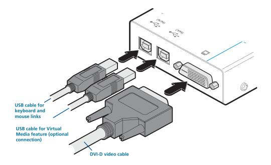
Figure 3-3. Connecting the video and USB cables
