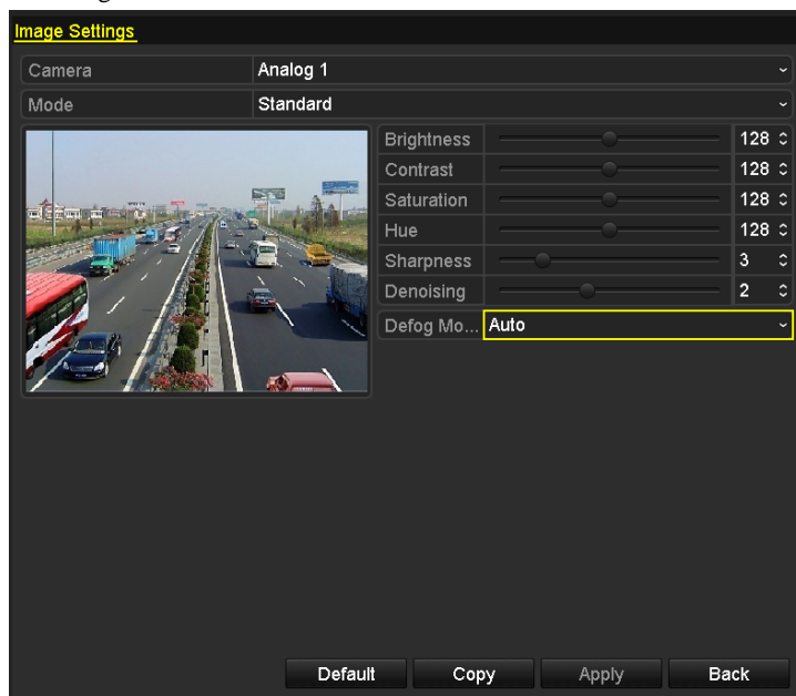
Figure 12. 5 Image Settings Interface for Analog Camera Connected to DS-9200 HWI-ST Series
