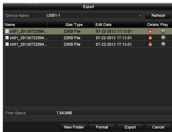
Figure 7.27 Checkup of Picture Export Using USB Flash Drive
