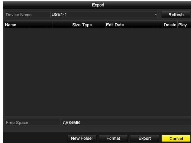
Figure 7. 17 Export Video Clips Using USB Flash Drive
