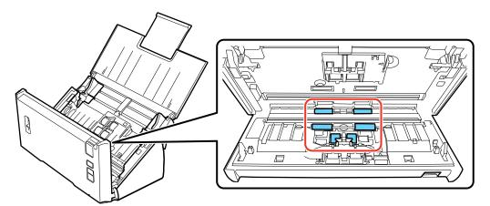
6. Wipe off any stains on the pickup rollers.
