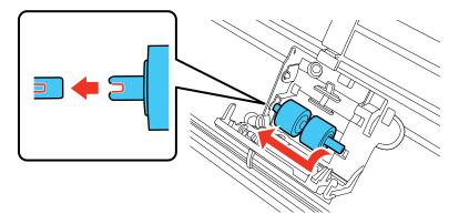
8. To install the new upper pickup roller, align the notches on the roller and slide it to the left. Make sure the smaller roller is on the bottom.
