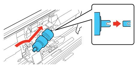
15. While applying gentle pressure on the separation roller, close the separation roller cover.
