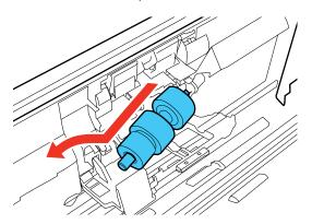
12. Pull the release tab on the separation roller and remove it from the spindle.
