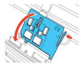
**Caution:** Do not place too much force on the arm inside the cover when replacing the pickup roller.
