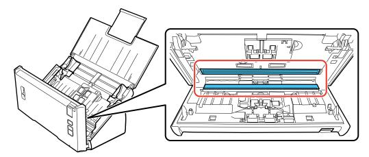
**Note:** If the glass surface is stained with grease or some other hard-to-remove material, use a small amount of glass cleaner on a soft cloth to remove it. Wipe off all remaining liquid.
