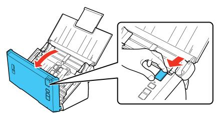
5. Use a soft, dry cloth to wipe off any stains on the rollers inside the scanner cover.
