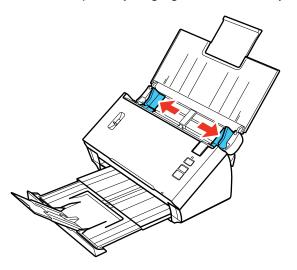
4. Load one card horizontally in the input tray as shown, sliding it in until it meets resistance. Make sure the printed side is facedown with the top facing into the scanner.
