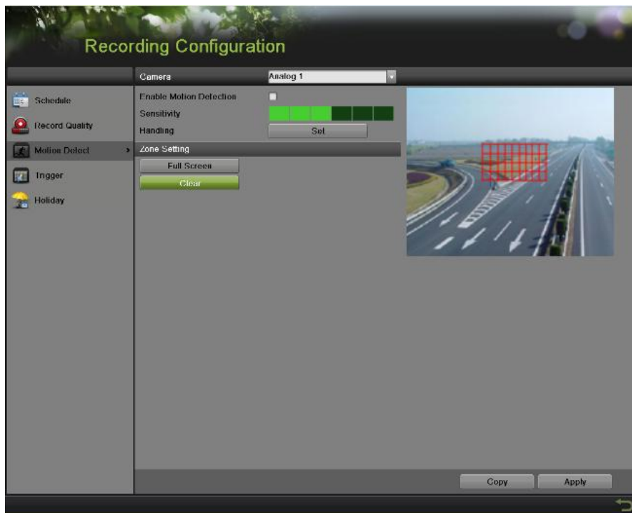
Figure 73 Motion Detection Settings Menu
