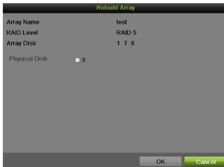
Figure 104 Rebuild Array Interface
