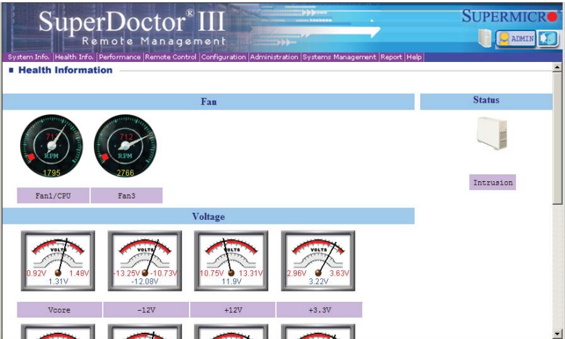
Figure 5-5. SuperDoctor III Interface Display Screen (Health Information)
