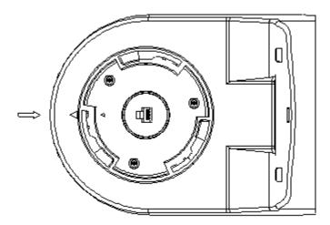
Insert the cables (Network) through the mounting plate and connect to the camera. Then use the little strap in bundled accessory to fasten the network cable.
