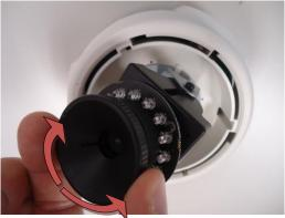
Remove the lens focus tuner.
