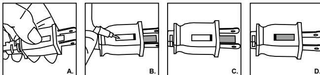
Risk of fire. Do not replace attachment plug. Contains a safety device (fuse) that should no be removed. Discard product if the attachment plug is damaged.
