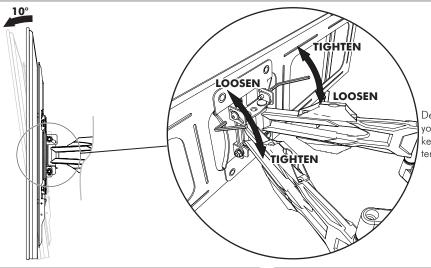
Depending on the weight of your display, you may need to use the supplied allen key to tighten and loosen the screws for tilt tension adjustment.
