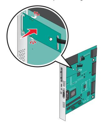
Connect the ISP solution interface cable into the receptacle of the system board.
