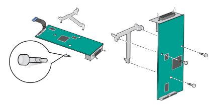
**5** Use the provided screw to attach the ISP solution to the system board cage.
