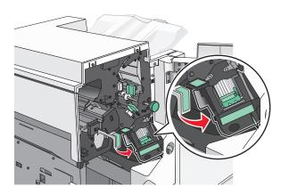
**3** Lower the latch of the staple cartridge holder, and then pull the staple cartridge holder out of the printer.
