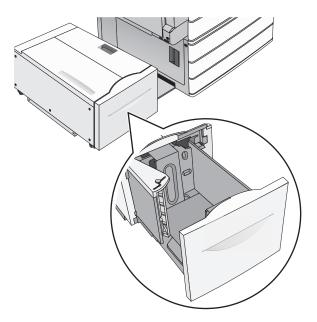
**2** Adjust the width guide as necessary.
