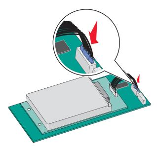
To install a printer hard disk directly on the system board:
