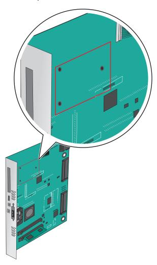
Note: If an optional ISP is currently installed, then the printer hard disk must be installed onto the ISP.
