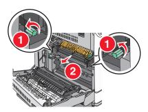
3 Firmly grasp the jammed paper on each side, and then gently pull it down and out.
