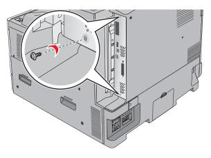
2 Pull the system board forward to remove it.
