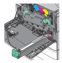
Rotate the release lever counterclockwise to open the cover.
