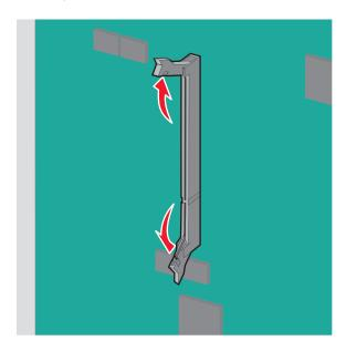
Align the notch on the memory card to the ridge on the connector.
