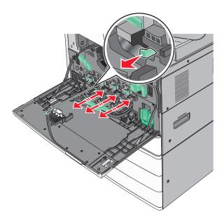
Slide the printhead wipers back into place.
