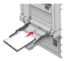
**Warning—Potential Damage:** Pulling the paper out, without pushing the paper pick tab first, may cause jams or the paper pick tab to break.
