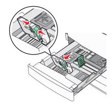
**3** Squeeze and then slide the length guide to the correct position for the paper size loaded.
