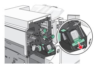
**4** Use the metal tab to lift the staple guard, and then remove any jammed or loose staples.
