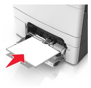
**4** Slide the paper guide until it rests lightly against the edge of the paper stack.
