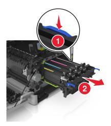
Remove the used developer unit.
