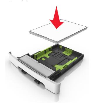
• Make sure the guides in the tray or the multipurpose feeder are properly positioned and are not pressing tightly against the paper or envelopes.
