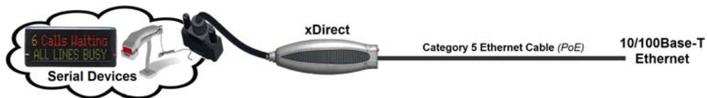
Figure 3-1 xDirect with PoE Connected to a Serial Device and Network
